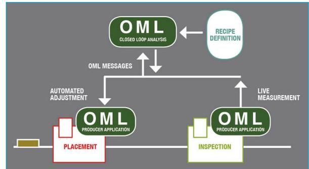
Figure 6: Closed-loop line control using OML.
