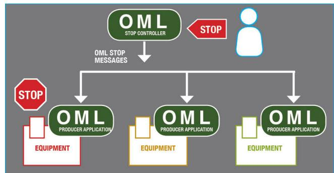
Figure 2: Poka-yoke execution using the bidirectional OML standard.
