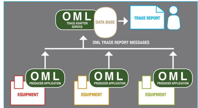
Figure 4: OML-based material traceability.
