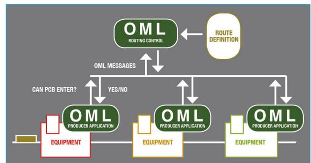
Figure 5: Bidirectional control for routing enforcement.
